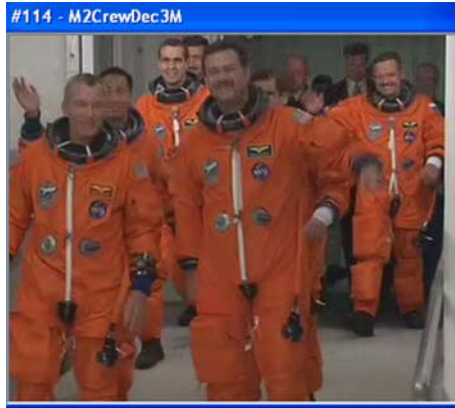
FIGURE 10: Transcoded H264 to MPEG-2 video and decrypted. H264 QP video of 26, and MPEG-2 Bitrate of 3 Mbps.
